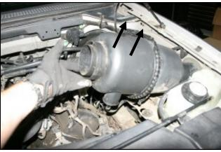
**3.** Lift straight up on the outlet side of the air filter canister to remove it from it's locating grommets. Next, pull it towards the engine to dislodge it from the inner fender well.
