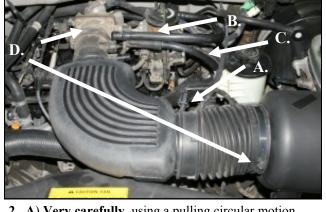
2. A) <u>Very carefully</u>, using a pulling circular motion, remove the air intake temperature sensor from the air intake tube. B) Disconnect the upper hard plastic tube from the air intake tube. C) Disconnect the crankcase breather at the intake tube and the valve cover, and remove it from the vehicle. D) Loosen two hose clamps and remove the air intake tube from the vehicle.
