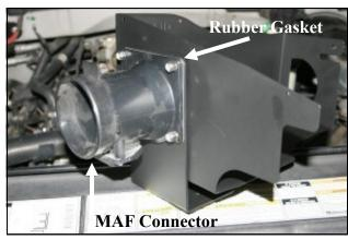
7. Attach the MAF bracket (#6), rubber gasket (#18), and factory MAF sensor housing to the Cold Air Dam (CAD) using four 1/4-20x7/8" hex bolts (#15), and 1/4" Nylock nuts (#17), as shown. Make sure that the MAF sensor connector is on the bottom when assembly is complete. Refer to the line drawing above for reference.
