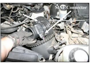
4.Unlatch the clamp on the canister to separate the two halves. Once separated, remove the factory air filter.
