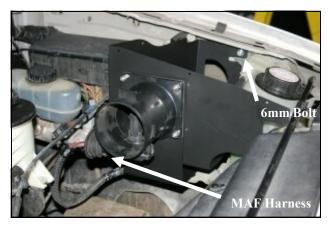
10. Install the CAD assembly into the vehicle using two 1/4-20x7/8" bolts (#15), four 1/4" flat washers (#16), one MAF backing plate (#19), and two 1/4" nylock nuts (#17). Leave the two bolts slightly loose for now for final adjustment. Refer to the line drawing on page 1 for reference. Next, reinstall the 6mm bolt thru the CAD, radiator overflow tank, and into the fender well. Reconnect the MAF sensor wiring harness.
